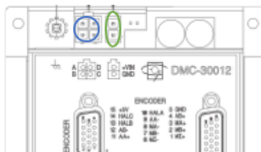
Figure 23. Location of the female 4-pin (blue) and 2-pin (green) ports on the Motion Controller
