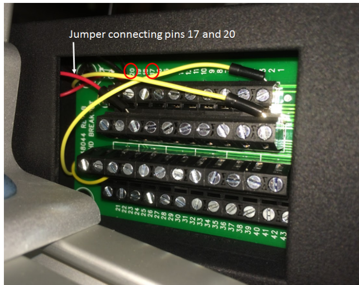
Figure 18. Jumper connection between ports 17 and 20 on the 44-pin Adapter
